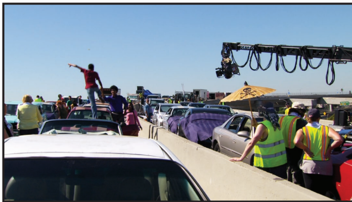
1.8 Eye in the sky. The Oculus mount on a crane extended the camera above the dancers and moved quickly with them via remote control. ( La La Land )
