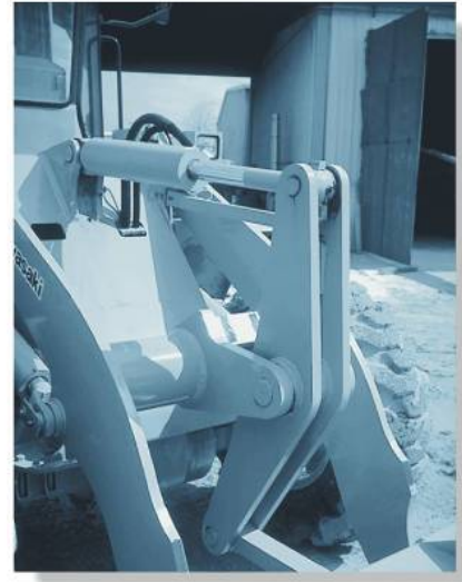
Many machine elements are pin connected in order to enable free rotation at their connections. These supports exert a force on a member, but no moment.
