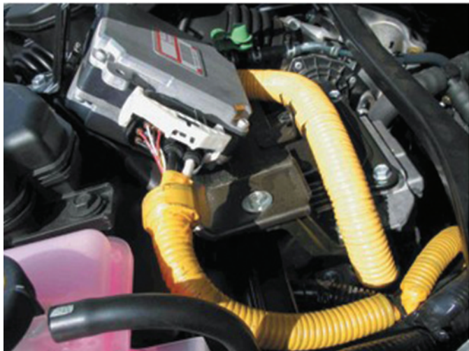
FIGURE 1-1b The yellow cable is part of the electric power steering system on a Toyota/Lexus vehicle.
