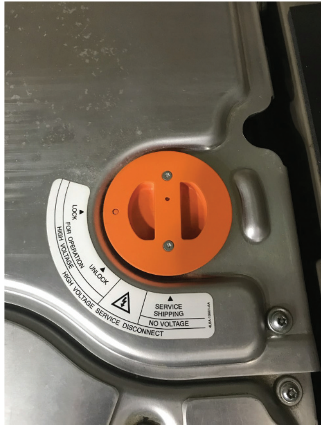
FIGURE 1-18 The manual disconnect on this Ford battery contains a fuse and safety interlock.
