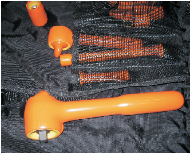
FIGURE 1-17 Insulated tools, such as this socket set, provide an additional margin of safety to the service technician when working around HV components and systems.
