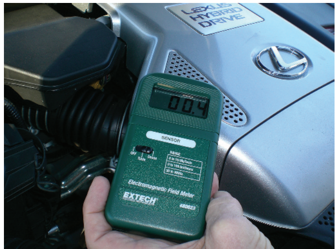
FIGURE 1-13 The radiation emitted from a hybrid electric vehicle is very low and is being measured in units of milligauss.
