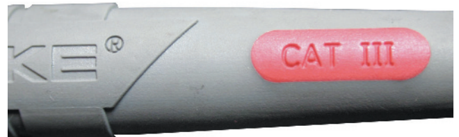
FIGURE 1-15 The meter leads should also be CAT III rated when checking voltages on an electric or hybrid electric vehicle.
