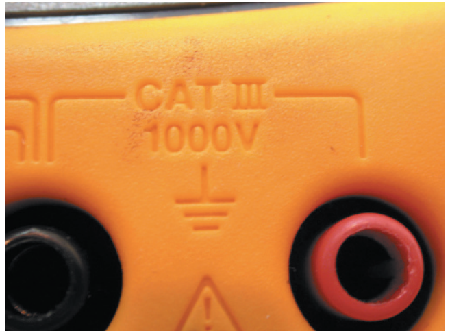
FIGURE 1-14 Use only a meter that is CAT III rated when making electrical measurements on an electric or hybrid electric vehicle.
