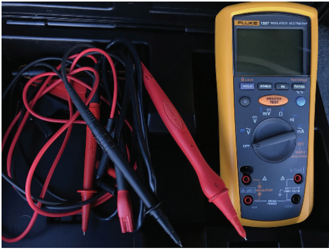
FIGURE 1-16 The Fluke 1587 is an example of an insulation tester that is able to test the HV circuit insulation to 1,000 volts. The resistance between the HV circuit and ground should be higher than one million ohms (1.0–22.2 MΩ).
