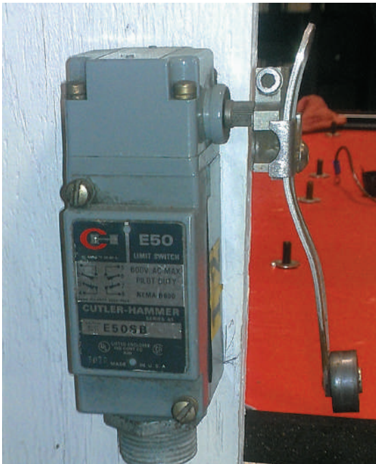
FIGURE 1-11 A limit switch.
