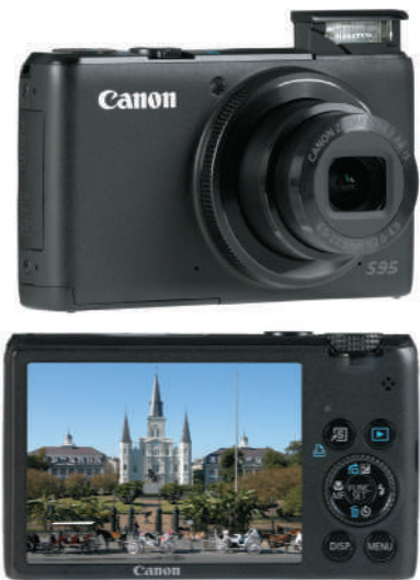
Figure 1-7 With a digital camera, you can view photographed images immediately through a small screen on the camera to see if the photo is worth keeping.
