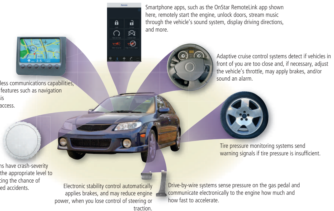
Figure 1-4: Some of the embedded computers designed to improve safety, security, and performance in today's vehicles
