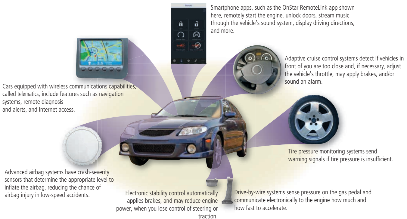
Figure 1-4: Some of the embedded computers designed to improve safety, security, and performance in today's vehicles
