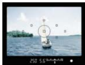
Aperture settings appear on a camera's lens aperture ring (shown above), in the viewfinder (below left), or as data-panel readout (below right). Here, the camera is set to f/5.6.
