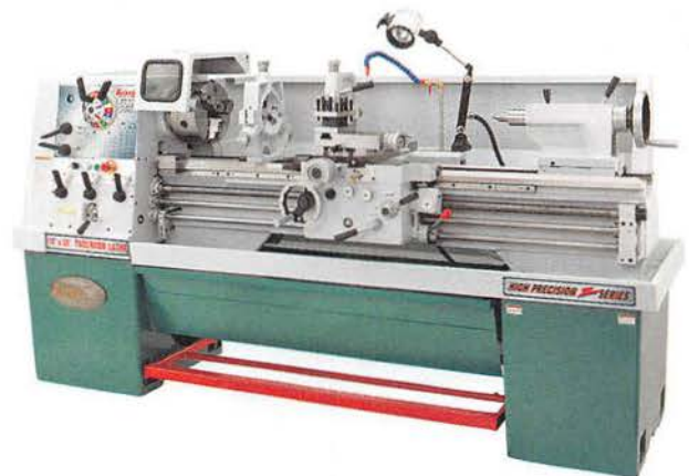
Figure 1-7. A modern lathe featuring chuck safety guard, foot brake, coolant system, inch/metric dials, and a universal gearbox capable of cutting inch, metric, and diametral threads. Except those tools that perform nontraditional machining operations, all machine tools have evolved from the lathe.
