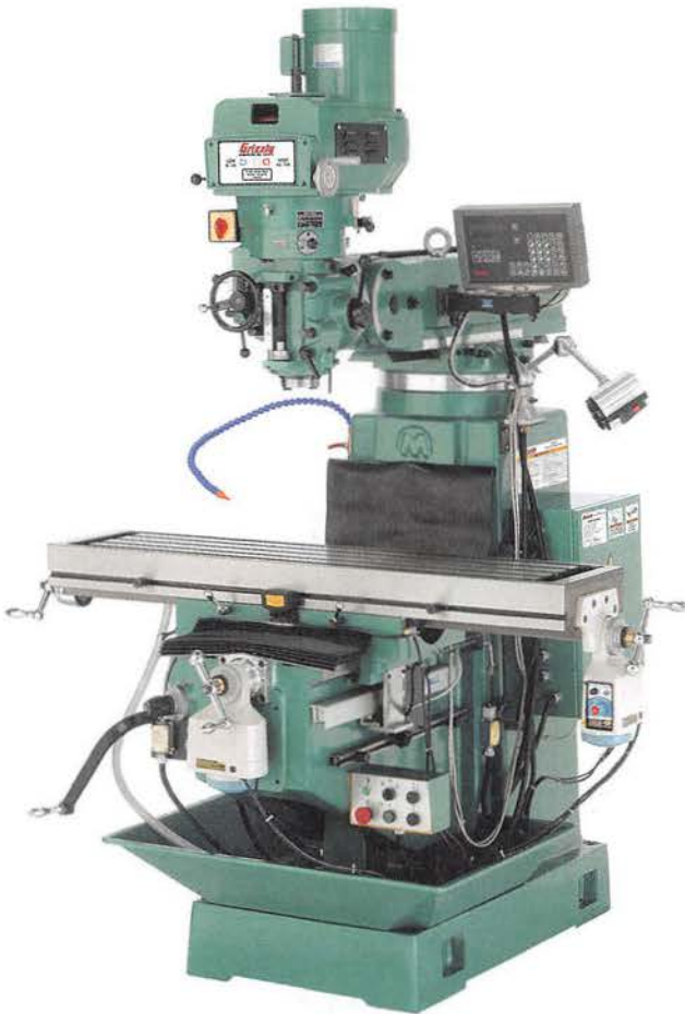
Figure 1-14. A modern milling machine featuring power feed, variable speed controls, an automatic stop function, coordinate display, and selectable resolution up to one micrometer.
