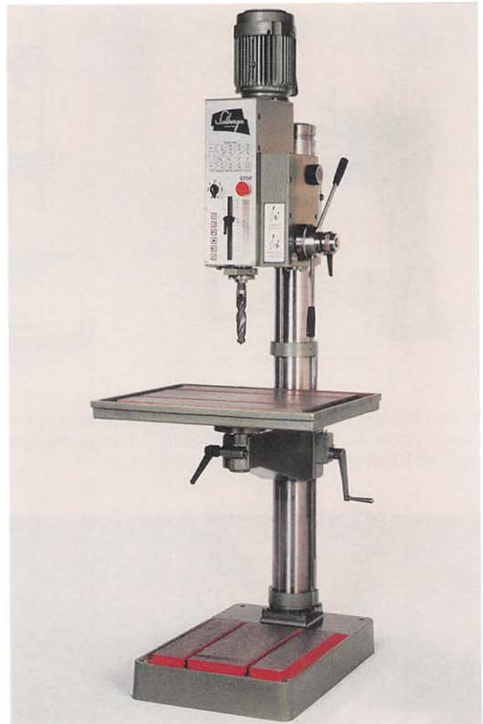
Figure 1-10. A typical 20" variable-speed gearhead drill press with power feed. It can drill holes up to 1 1/2" in diameter in cast iron.
