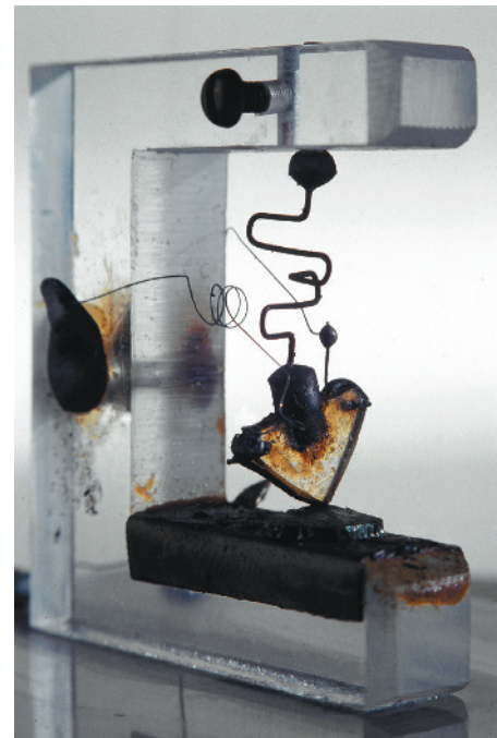
FIG. 1.3 The first transistor. SSPL/Getty Images
