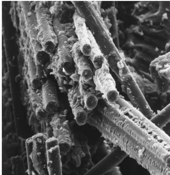
FIGURE 1.14 Example of a fiberglass composite composed of microscopic-scale reinforcing glass fibers in a polymer matrix. (Courtesy of Owens-Corning Fiberglass Corporation.)
