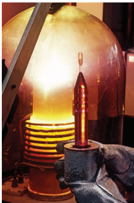
FIGURE 1.6 An yttrium-aluminum-oxide ( Y_3Al_5O_{12} or YAG) crystal grown over a period of 21 days for use in laser rods. (James L. Amos / Science Source.)
