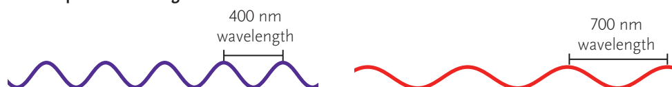
FIGURE 1.3 The electromagnetic spectrum. (a) The electromagnetic spectrum ranges from gamma rays to radio waves; visible light and the wavelengths used for photosynthesis occupy only a narrow band of the spectrum. (b) Examples of wavelengths show the difference between the longest and shortest wavelengths of visible light.
