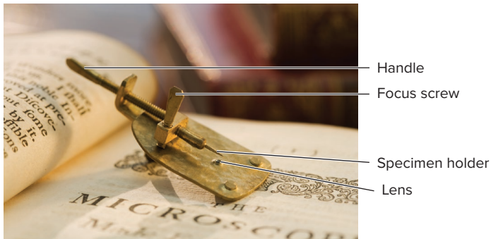
FIGURE 1.1 Model of van Leeuwenhoek's Microscope The original made in 1673 could magnify an object almost 300 times. The object is brought into focus with the adjusting screws. Tetra Images/Alamy Stock Photo
