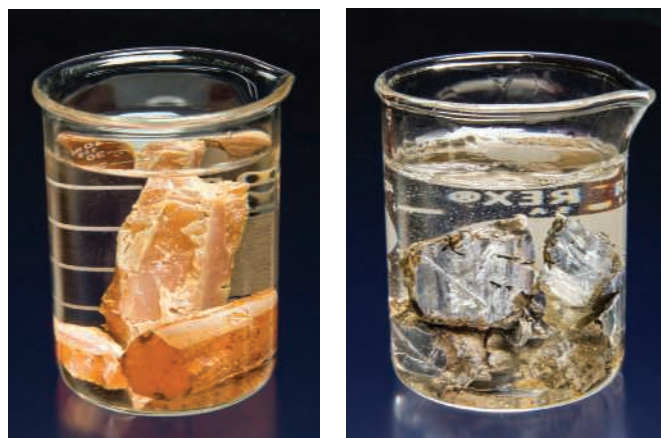
Elements: yellow phosphorus in water (left) and shiny potassium under oil (right).
