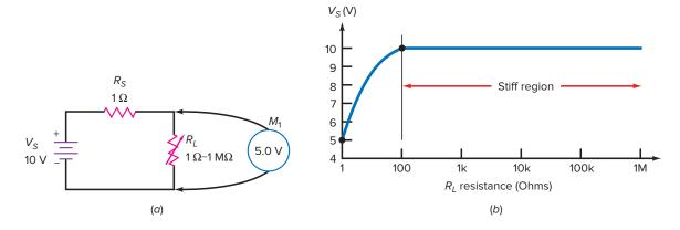
load voltage, regardless of how small or large the load resistance is. With an ideal voltage source, only the load current changes when the load resistance changes.
