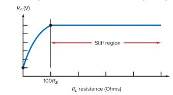
with a stiff voltage source. As long as the load resistance is greater than  $100R_S$ , the voltage source is stiff. When the load resistance equals this worst-case value, the calculation error from ignoring the source resistance is 1 percent, small enough to ignore in a second approximation.
