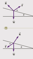
Figure CS1.1 The forces acting on (a) the shearer and (b) the sheep, where \mathbf{F} = dragging force, \mathbf{R} = ground reaction, \mathbf{W} = weight, \theta = angle of inclination.
