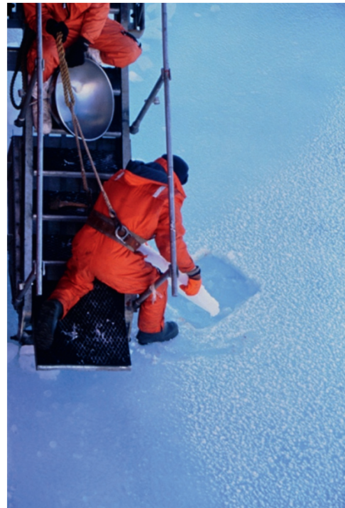
Figure 1.1 Sampling of 0.05 m thick sea ice in the Baffin Bay in May 1998 by the author (Shokr) using a gangway lowered from an icebreaker (photo by K. Asmus, Canadian Ice Service).
