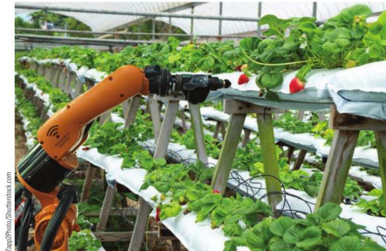
Figure 1-9: Robot used to detect weeds and spray chemicals
