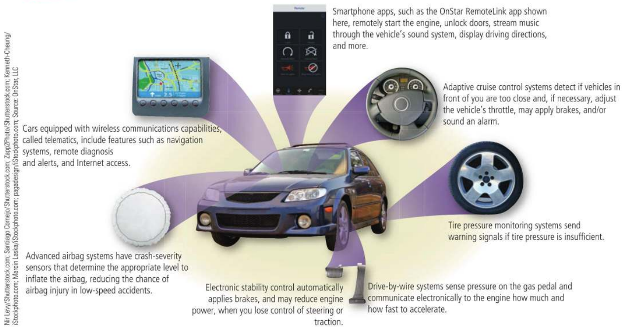
Figure 1-4: Some of the embedded computers designed to improve safety, security, and performance in today's vehicles
